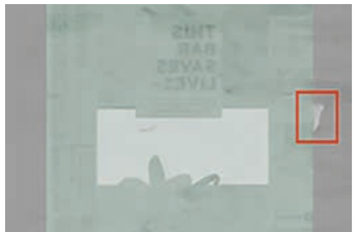
The PrintSTAR system simultaneously checks the front and back of the substrate in a superimposed image for register errors and other defects
