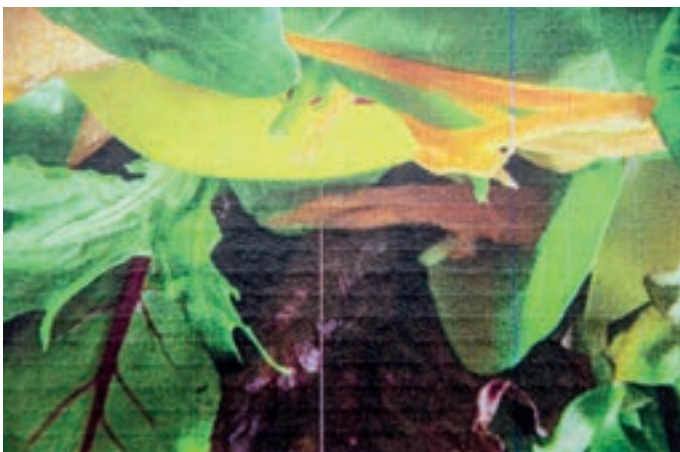
Streaking due to clogged nozzles is one of the most common printing defects in digital printing
