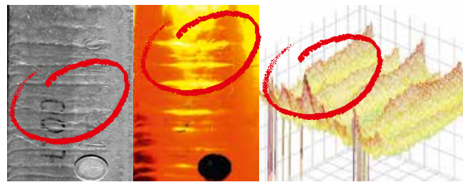
Sophisticated 2D inspection & innovative 3D technology combined – reliable defect detection on the slab surface
